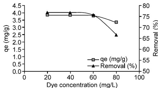
Fig. 10: The effect of dye concentration on adsorption efficiency
