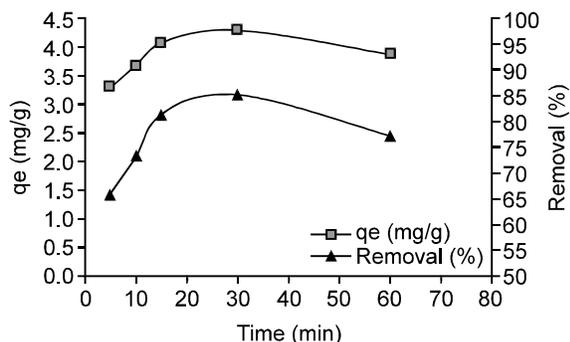
Fig. 9: The effect of contact time on adsorption efficiency
