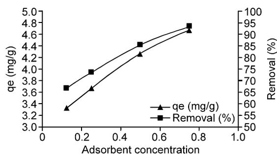
Fig. 11: The Effect of Adsorbent (ESM) concentration on dye efficiency
